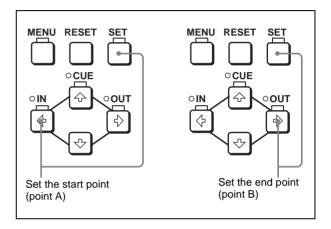
The time code of the current playback position is set as point A or point B.
